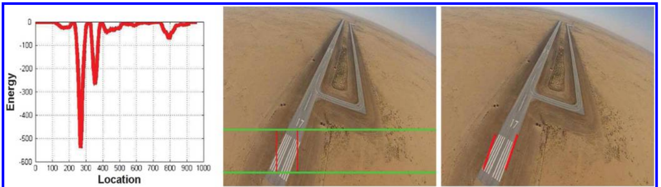
Fig. 5 Energy profile and candidate line segments outlining the runway.
