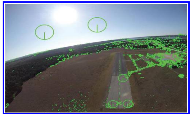
Fig. 8 Feature points detected by Harris detector.
